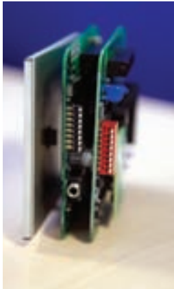
The aluminium backing plate was re-designed to also house the RF circuitry
